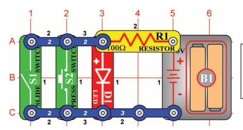
Build the circuit at left and test the combinations of the slide switch (S1) and press switch (S2). If you compare it to the OR circuit in Project #47, you can see the LED lights in the opposite combinations of that circuit. Hence, we refer to it as a <u>NOR</u> circuit (short for "NOT this OR that"). Like the OR and AND, it is an important building block in computers.
